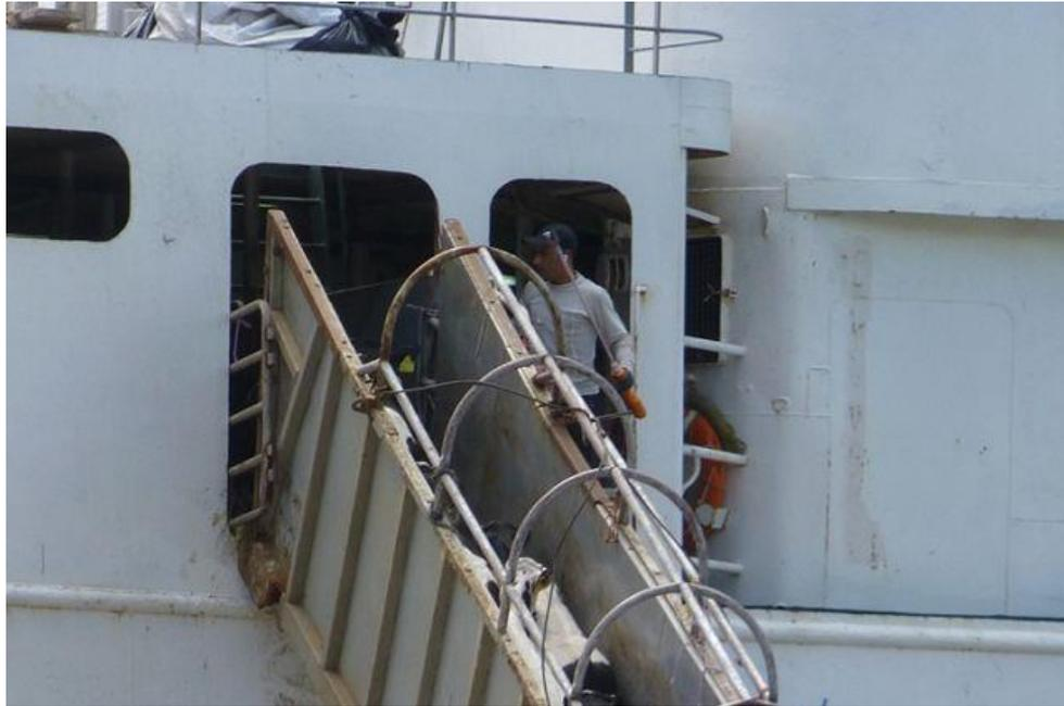
*Vessels' entry is very dark, small calves loaded via a very steep ramps exceeding 20°*
