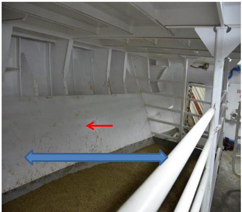
*On the left: good practice – the side wall is covered (red arrow) and the pen facilities are not adjacent to the ship's wall. That facilitates the inspection and access to the animals in the enclosures.*
